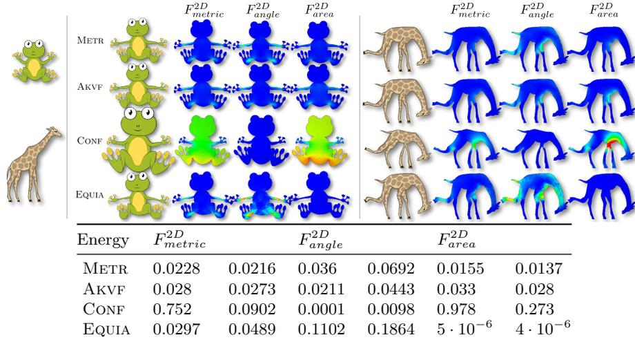
**Fig. 5.** 2D Energy Evaluation. Two initial models (left) are deformed using the same boundary constraints for the different energy types. The plots visualize color coded local errors. The CONF error plots for the frog are downscaled to 75% size. The table gives total errors for each method and each model (frog left / giraffe right column).
