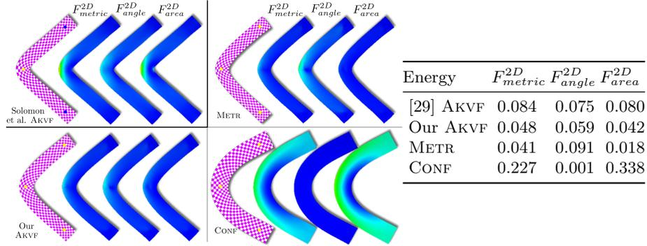
**Fig. 6.** AKVF Comparison. A symmetric strip deformation is used to evaluate our energies and compare them to the original AKVF formulation [29] that uses no energy based smoothing and only soft constraints. The color coded images visualize local error components, which are all scaled equally.
