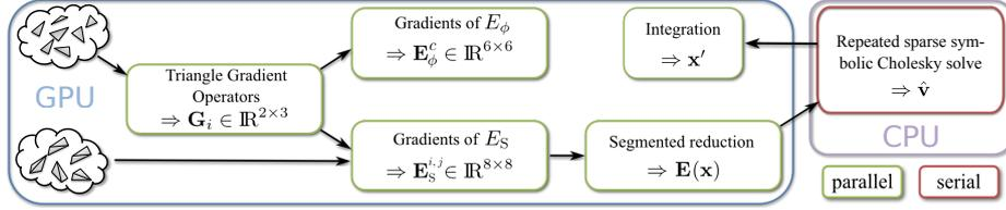
**Fig. 4.** GPU Pipeline. We use the GPU to setup linear systems and perform vector field integration. The linear systems are solved on the CPU using an efficient sparse solver. Operations marked (●) are performed in parallel on the GPU.
