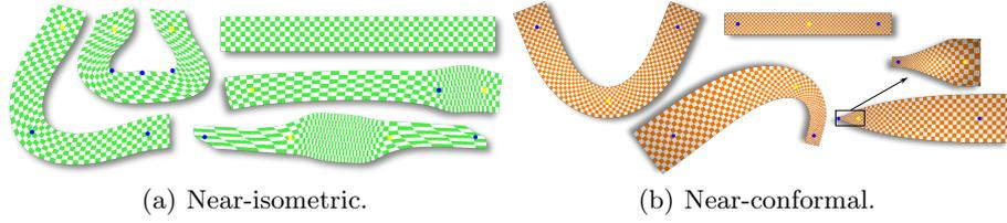
**Fig. 1.** 2D Deformation Examples. On the straight strip some vertices were fixed ( $\bullet$ ) while some vertices were moved ( $\circ$ ) (all models have the same scale). The deformations are generated by AMAP (8) and ACAP (12) vector fields. Note the approximate length preservation in (a), and the preservation of angles and the area deviation in (b).
