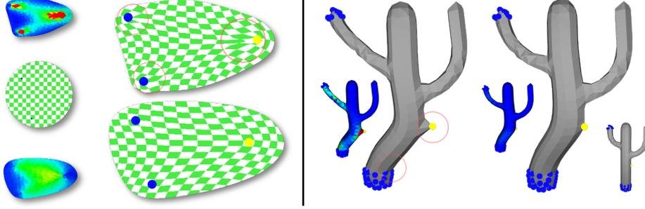
**Fig. 3.** Smoothness Energy. In  $2d$  (left) and  $3d$  (right) minimizers of the generalized metric energy are discontinuous near user constraints (fixed  $\bullet$  and handle  $\bullet$  vertices) leading to the highlighted local discontinuous deformations (small images show metric distortions, see Section 6). The smoothness energy term yields smooth vector fields and therefore smooth deformations. Note that both interior (left) and boundary vertices (right) can be constrained.
